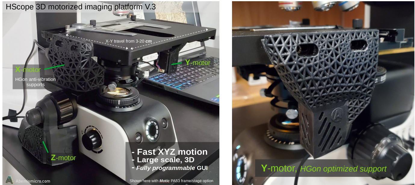
Figure 1. Left, Motic PA53 HScope with V.3 XYZ motors. Right, closeup of Y-axis ultra-light, anti-vibration motor support.
